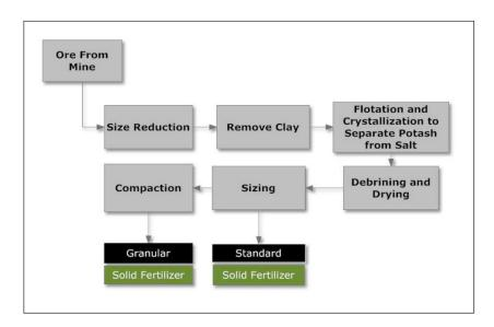
$Figure \ i-Simplified \ flow \ diagram \ for \ potash \ flotation \ and \ crystallization \ milling \ methods \ used \ at \ Rocanville.$
